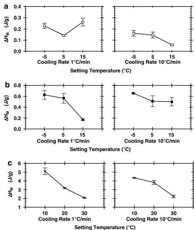
**Fig. 7** Effect of cooling rate and setting temperature on  $\Delta H_M$  for organogels developed at 0.5% (a), 1% (b), and 3% (c) CW concentration in SFO.  $\Delta H_M$  is defined in the text
