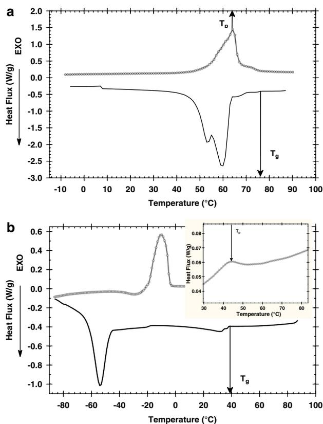
**Fig. 2** Cooling (solid line) and heating (dotted line) thermograms for CW (a) and a 3% CW dispersion in SFO (b). The insert is the enlarged section between 30 and 80 °C for the heating thermogram, showing the endotherm for the CW dispersion.  $T_p$  and  $T_g$  are defined in the text
