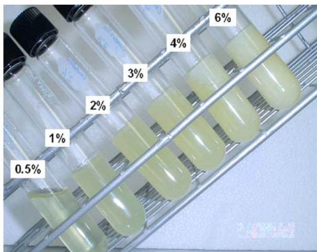
**Fig. 4** Visual appearance of organogels developed at 25 °C as a function of CW concentrations in SFO
