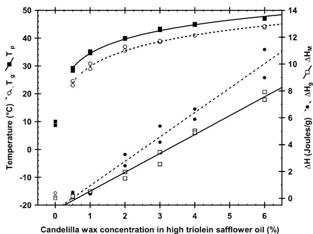
**Fig. 3** Behavior of the thermal parameters that characterized organogel development ( $T_g$ ,  $\Delta H_g$ ) and melting ( $T_p$  and  $\Delta H_M$ ) as a function of CW concentration in SFO.  $T_g$ ,  $\Delta H_g$ ,  $T_p$ , and  $\Delta H_M$  are defined in the text
