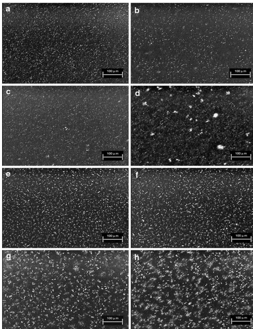
**Fig. 10** Polarized light microphotographs (50× magnification) of CW organogels at 7 days of storage at  $T_{\text{set}}$  of 5 °C (a, c) and 25 °C (b, d). 1% CW (a, b) and 3% CW (c, d)
