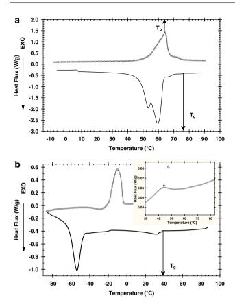
**Fig. 2** Cooling (*solid line*) and heating (*dotted line*) thermograms for CW (**a**) and a 3% CW dispersion in SFO (**b**). The insert is the enlarged section between 30 and 80 °C for the heating thermogram, showing the endotherm for the CW dispersion.  $T_{\rm p}$  and  $T_{\rm g}$  are defined in the text
