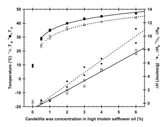
**Fig. 3** Behavior of the thermal parameters that characterized organogel development  $(T_{\rm g}, \Delta {\rm H_g})$  and melting  $(T_{\rm p} \ {\rm and} \ \Delta {\rm H_M})$  as a function of CW concentration in SFO.  $T_{\rm g}, \Delta {\rm H_g}, T_{\rm p}$ , and  $\Delta {\rm H_M}$  are defined in the text
