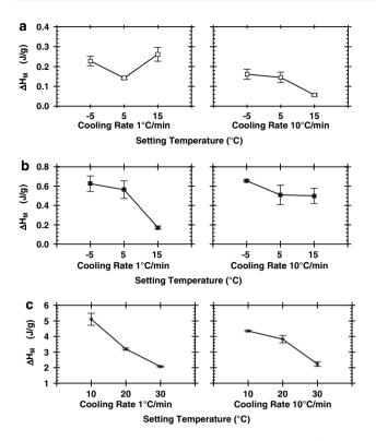
**Fig. 7** Effect of cooling rate and setting temperature on  $\Delta H_{\rm M}$  for organogels developed at 0.5% (a), 1% (b), and 3% (c) CW concentration in SFO.  $\Delta H_{\rm M}$  is defined in the text
